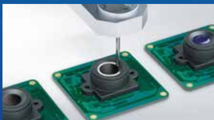
Capable of adhesive application on optical components
