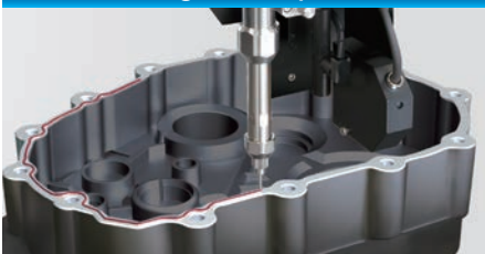
Dispensing CIPG on Engine Component
