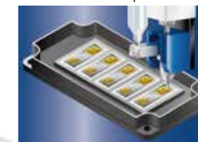
Dispensing solder paste on IGBT modules
