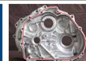
Liquid gasket sealing of an engine parts
