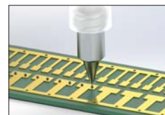
Solder paste dispensing to lead frame
