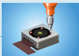
Dispensing UV on Camera Module
