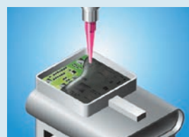
Pressure Sensor Potting
