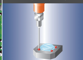
UV glue dispensing to Optical pickup
